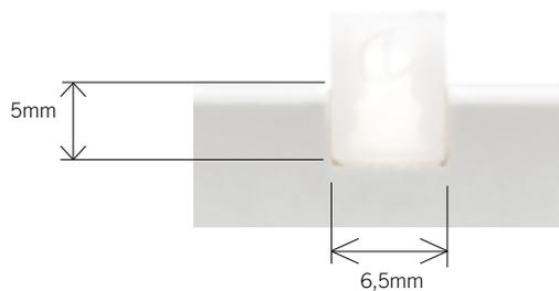
The **APEX 86 HI** profile design can be used also for semi-recess installation, guaranteeing a 180° light projection.
