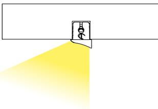
**LAB** has a special eyelid designed to eliminate the glare effect. Light projection is screened from the user and directed towards the inside of the lit compartment.
