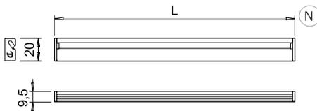
**BLADE-IN HI** is designed for recessed installation in a blind or through milled groove which is 20mm wide and 9,5mm deep.
